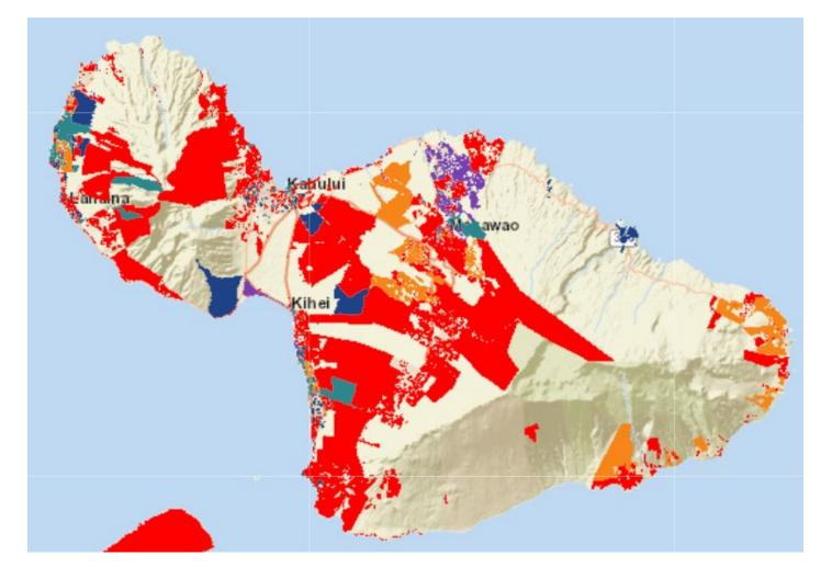
DG PV penetration on some circuits exceed 300% DML
